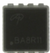
AON6411 Alpha & Omega Semiconductor Inc. MOSFET P-CH 20V 47A 8DFN
