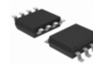
24LC64T-E/SN Microchip Technology IC EEPROM 64KBIT 400KHZ 8SOIC
