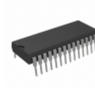
AT28HC256-90PI Microchip Technology IC EEPROM 256KBIT 90NS 28DIP
