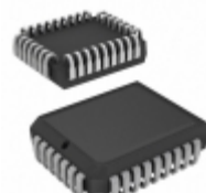
AT28HC256-90JU-T Microchip Technology 90NS, PLCC, IND TEMP, GREEN
