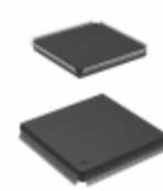
A54SX32A-1CQ208B Microsemi Corporation IC FPGA 174 I/O 208CQFP
