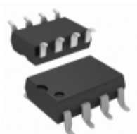
6N138S-TA1 Lite-On Inc. OPTOISO 5KV DARL W/BASE 8SMD
