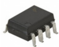
6N138SD Fairchild/ON Semiconductor OPTOISO 2.5KV DARL W/BASE 8SMD
