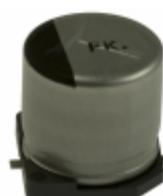
EEV-FK1C681GP Panasonic Electronic Components CAP ALUM 680UF 20% 16V SMD
