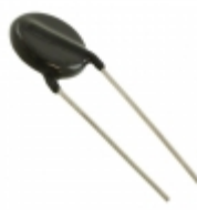
ERZ-E14A511 Panasonic Electronic Components VARISTOR 510V 10KA DISC 16.5MM
