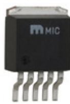
MIC5209-3.0YU-TR Microchip Technology IC REG LDO 3V 0.5A TO263-5
