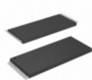
AT29BV010A-25TC Microchip Technology IC FLASH 1MBIT 250NS 32TSOP
