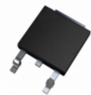
IRLR3802TRLPBF Infineon Technologies MOSFET N-CH 12V 84A DPAK
