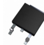
IRLR3717TRRPBF Infineon Technologies MOSFET N-CH 20V 120A DPAK
