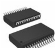
PIC24FJ32GA002-I/SS Microchip Technology IC MCU 16BIT 32KB FLASH 28SSOP
