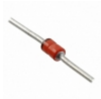
MXLP4KE68A Microsemi Corporation TVS DIODE 58.1VWM 92VC DO41
