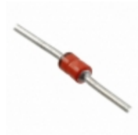
MXLP4KE6.8AE3 Microsemi Corporation TVS DIODE 5.8VWM 10.5VC DO41
