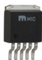
MIC29371-5.0WU Microchip Technology IC REG LDO 5V 0.75A TO263-5
