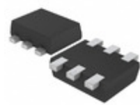
EMX52T2R Rohm Semiconductor TRANS 2NPN 50V 0.1A EMT6
