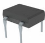
DBL157G C1G TSC (Taiwan Semiconductor) BRIDGE RECT 1PHASE 1KV 1.5A DBL
