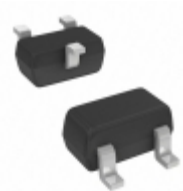
MMBD4448HT-TP Micro Commercial Co DIODE GEN PURP 80V 250MA SOT523
