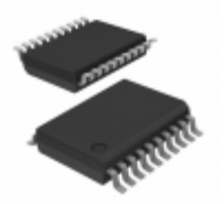
DSPIC33FJ06GS101A-I/SS Microchip Technology IC MCU 16BIT 6KB FLASH 20SSOP
