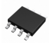
BR24C08-RDS6TP Rohm Semiconductor IC EEPROM 8KBIT 100KHZ 8TSSOP
