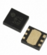
XC6121A443ER-G Torex Semiconductor Ltd IC WATCHDOG TIMER 6-USP
