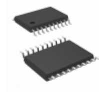
ADG3300BRUZ-REEL Analog Devices Inc. IC XLATOR 8CH 1.2/5.5V 20-TSSOP
