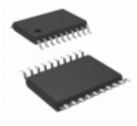
ADG3300BRUZ Analog Devices Inc. IC XLATOR 8CH 1.2/5.5V 20TSSOP
