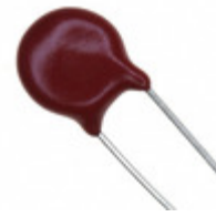
V18ZC1 Littelfuse Inc. VARISTOR 18V 250A DISC 7MM
