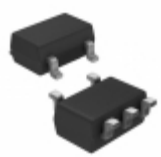
S-1000C45-M5T1G SII Semiconductor Corporation IC VOLT DETECTOR 45V SOT23-5
