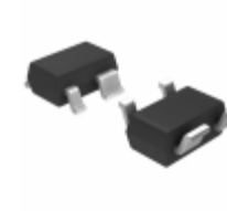
S-1000C46-N4T1G SII Semiconductor Corporation IC VOLT DETECTOR 46V SC-82AB
