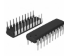
PIC24FJ32MC101-E/P Microchip Technology IC MCU 16BIT 32KB FLASH 20DIP
