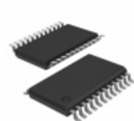
ATF22V10C-10XC Microchip Technology IC PLD 10MC 10NS 24TSSOP
