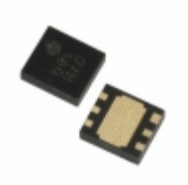
XC6122D525ER-G Torex Semiconductor Ltd IC WATCHDOG TIMER 6-USP
