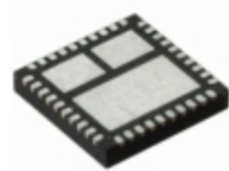
FDMF6823B Fairchild/ON Semiconductor MODULE DRMOS 55A 40-PQFN
