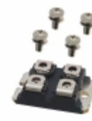
APT30F60J Microsemi Corporation MOSFET N-CH 600V 31A SOT-227
