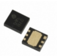
XC6122A432ER-G Torex Semiconductor Ltd IC WATCHDOG TIMER 6-USP
