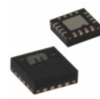
MIC2215-MMMYML-TR Microchip Technology IC REG LDO 2.8V 0.25A 16MLF
