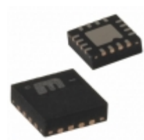
MIC2215-AAAYML-TR Microchip Technology IC REG LDO ADJ 0.25A 16MLF
