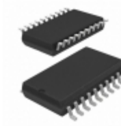
MC74LVX245M ON Semiconductor IC BUS TRANSCVR 8BIT 20SOEIAJ
