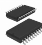
MC74LVX244DWR2G ON Semiconductor IC BUFF/DVR DUAL N-INV 20SOIC
