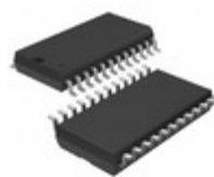
LTC1275ACSW#PBF ADI (Analog Devices, Inc.) IC A/D CONV 12BIT SAMPLING 24SOIC
