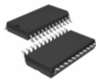
LTC1274ISW#TRPBF Linear Technology IC A/D CONV 12BIT W/SHTDN 24SOIC
