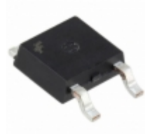
FDD5N50FTF_WS Fairchild/ON Semiconductor MOSFET N-CH 500V 3.5A DPAK
