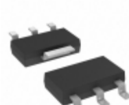
MCP1826ST-5002E/DB Microchip Technology IC REG LDO 5V 1A SOT223-3
