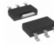
MCP1826ST-3302E/DB Microchip Technology IC REG LDO 3.3V 1A SOT223-3
