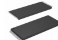
AT49LV002-90TI Microchip Technology IC FLASH 2MBIT 90NS 32TSOP
