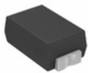
CDZT2RA7.5B Rohm Semiconductor DIODE ZENER 7.5V 100MW VMN2
