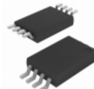
BR24C02-RDW6TP Rohm Semiconductor IC EEPROM 2KBIT 100KHZ 8TSSOP
