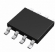
BR24C02-RDS6TP Rohm Semiconductor IC EEPROM 2KBIT 100KHZ 8TSSOP
