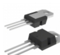
MIC39150-1.8WT Microchip Technology IC REG LDO 1.8V 1.5A TO220-3
