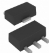
MCP1804T-C002I/MB Microchip Technology IC REG LDO 12V 0.15A SOT89-3
