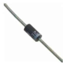
1N5950E3/TR13 Microsemi Corporation DIODE ZENER 110V 1.5W DO204AL
