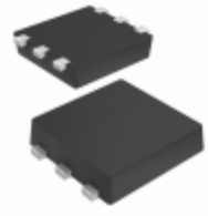
S-1112B35PI-L6UTFU SII Semiconductor Corporation IC REG LDO 3.5V 0.15A SNT6A
