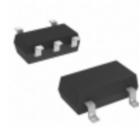
XN0155800L Panasonic Electronic Components TRANS 2NPN 20V 0.5A MINI5
