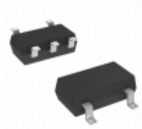
XN0150400L Panasonic Electronic Components TRANS 2NPN 20V 0.3A MINI5
