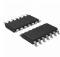
ALD4303SBL Advanced Linear Devices Inc. IC COMP VOLT CMOS OD QUAD 14SOIC
