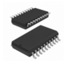
ALD4501SEL Advanced Linear Devices Inc. IC OSC TIMER QUAD 2MHZ 20SOIC
