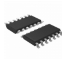
ALD4303ASBL Advanced Linear Devices Inc. IC COMP VOLT CMOS OD QUAD 14SOIC
