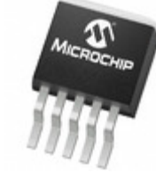
MCP1827-5002E/ET Microchip Technology IC REG LDO 5V 1.5A DDPAK
