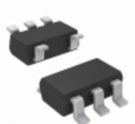
MCP1322T-31GE/OT Microchip Technology IC SUPERVISOR 3.1V SOT23-5
