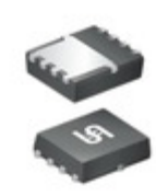
TSM038N03PQ33 RGG TSC (Taiwan Semiconductor) MOSFET N-CH 30V 78A 8PDFN
