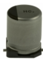
EEE-HC1E101P Panasonic Electronic Components CAP ALUM 100UF 20% 25V SMD
