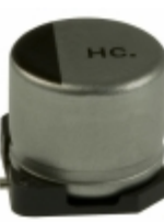
EEE-HC0J221XP Panasonic Electronic Components CAP ALUM 220UF 20% 6.3V SMD
