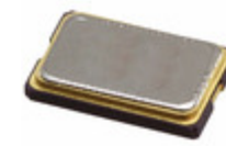
CX532Z-A5B3C5-70-25.0D18 Cardinal Components Inc. CRYSTAL 25.0000MHZ 18PF SMD
