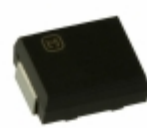
ECC-T3F330JG2 Panasonic Electronic Components CAP CER 33PF 3KV SL/GP SMD
