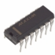
DS1801+ Maxim Integrated IC POT DUAL AUDIO TAPER 14DIP
