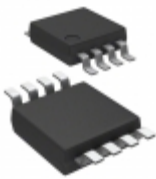
93C56AT-I/MS Microchip Technology IC EEPROM 2KBIT 2MHZ 8MSOP
